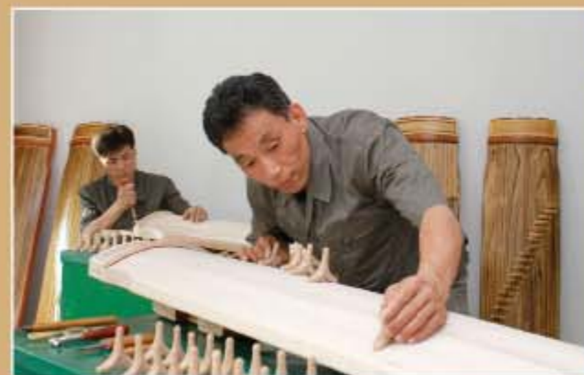
Base adjusting of kayagum 's bridges
